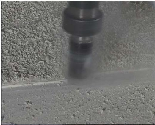
*Figure 7. High speed CNC milling of Robotically Applied Fairing Compound*
