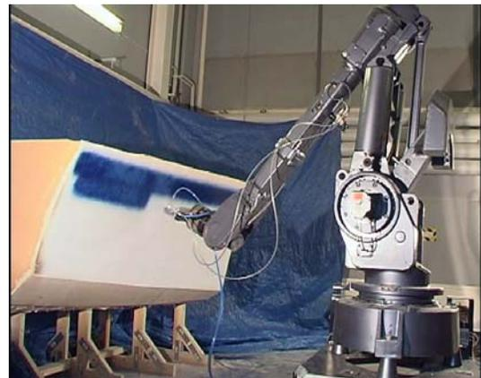
*Figure 9. Robotic spray system with HVLP gun*
