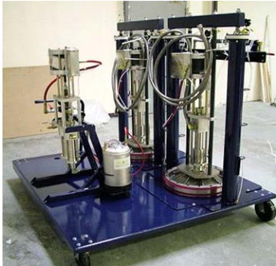
Figure 4. Plural Component Spray Pump System
