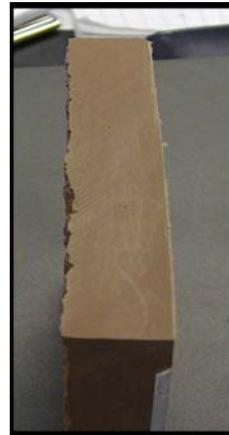
Figure 6. Cross-section of single-pass Robotically Applied Fairing Compound
