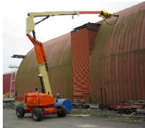
*Figure 11. Mobile Robot for Surface Preparation and Coatings Application*
