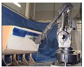
Figure 9. Robotic spray system with HVLP gun
