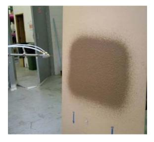
Figure 5. P.C. Spray tip applying single pass of Robotically Applied Fairing Compound
