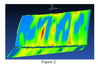
The data from the topographic image is processed further to create the ideal reference surface as represented in Figure 3. Control information is generated by the application software and then used to develop the tool path instructions for subsequent steps in the coatings application process. These steps include: Plural Component spraying of 100% Solids Fairing Material, CNC Milling of the Faired Surface, Robotic Sanding and Painting.
