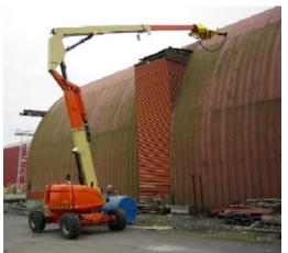
Figure 11. Mobile Robot for Surface Preparation and Coatings Application
