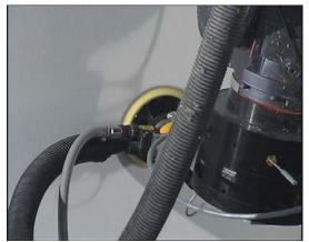
Figure 8. Robotic sanding with vacuum-throughhead sanding tool in single-head configuration
