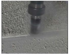
Figure 7. High speed CNC milling of Robotically Applied Fairing Compound
