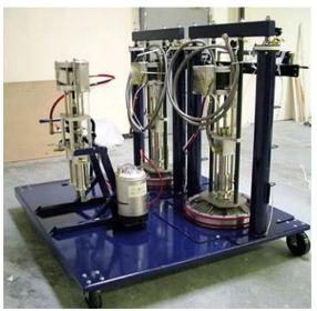
Figure 4. Plural Component Spray Pump System
