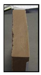
Figure 6. Cross-section of single-pass Robotically Applied Fairing Compound
