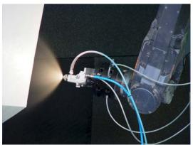
Figure 10. Robotic spray system with HVLP gun minimizes overspray for high transfer efficiency
